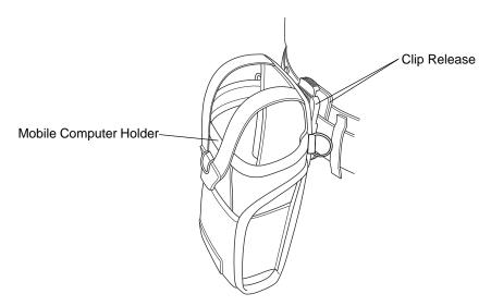
Figure 4-12 Attaching the Fabric Holster To a Belt
