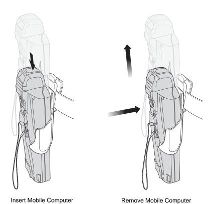
Figure 4-10 Insert and Remove the Mobile Computer
