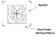
Figure 2-23 Centering Symbol in Aiming Pattern
