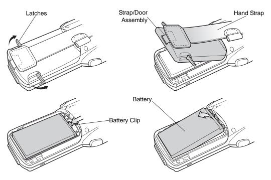
Figure 1-10 Main Battery Removal (MC3000S/R)
