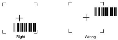
Figure 2-19 Bar Code not Centered in Aiming Pattern
