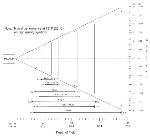
Figure 2-21 MC3000 Imager Decode Ranges
