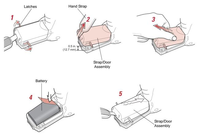
**Figure 1-6** *Main Battery Installation (MC3090G)*
