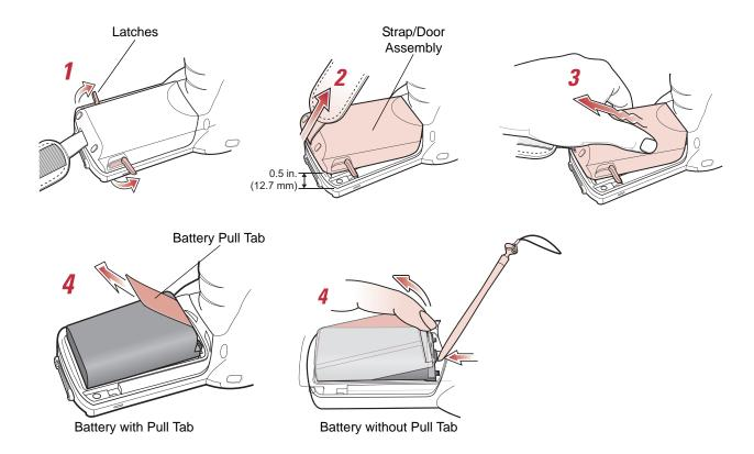
Figure 1-11 Main Battery Removal (MC3090G)
