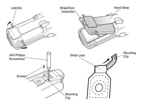
**Figure 1-12** Strap/Door Removal and Replacement (MC3000S/R)
