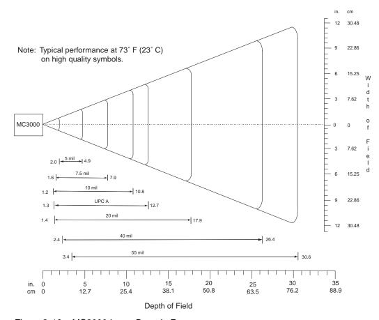
Figure 2-16 MC3000 Laser Decode Ranges
