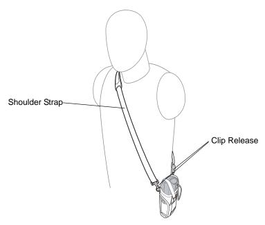
Figure 4-13 Attach the Fabric Holster To the Shoulder Strap
