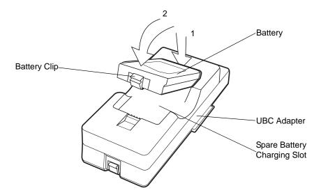
Figure 4-5 UBC Adapter Battery Insertion
