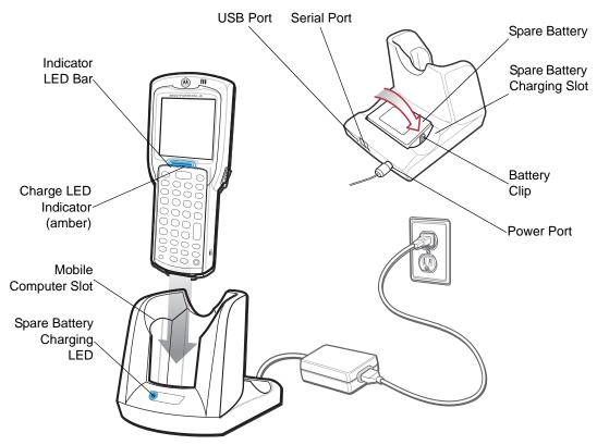
Figure 4-1 Single Slot Serial/USB Cradle
