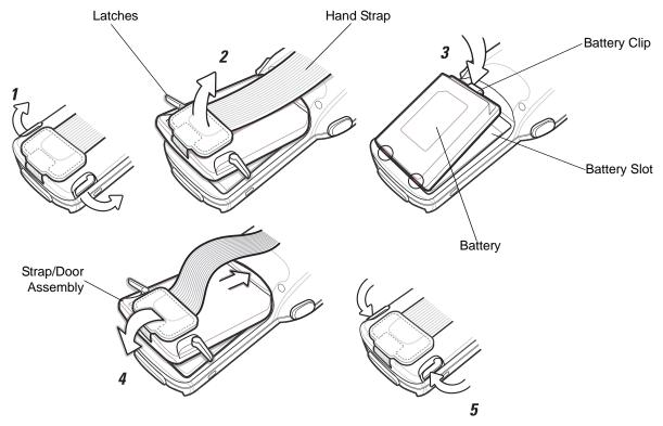
**Figure 1-5** *Main Battery Installation (MC3000S/R)*
