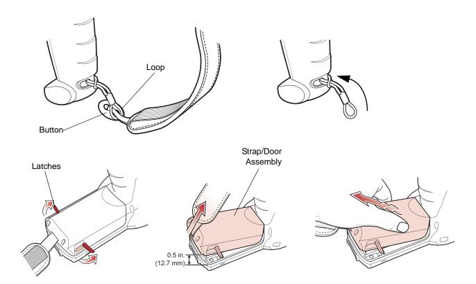
Figure 1-13 Strap/Door Removal and Replacement (MC3090G)
