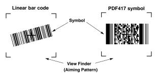
Figure 2-18 Centering Symbol in Aiming Pattern
