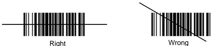
Figure 2-15 Laser Aiming
