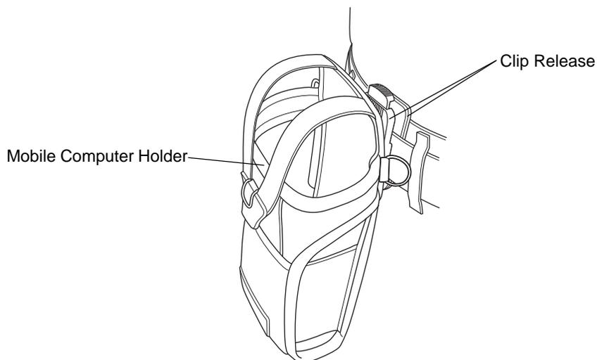
*Figure 4-12 Attaching the Fabric Holster To a Belt*
