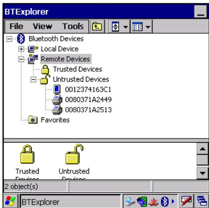
Figure 3-11 Discovered Devices Listed in Untrusted Folder
