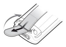
Figure 1-17 Slide Handstrap through Clip
