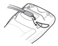
Figure 1-11 Insert Loop into Tether Point
