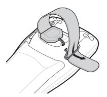
Figure 1-16 Slip End Through Loop
