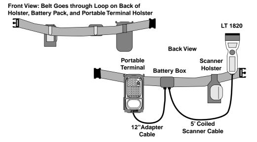
You can use either an alkaline battery, or a nickel-cadmium rechargeable battery, with an LT 1820 scanner. Low battery power is signaled by four short, high tone beeps, coupled with scanning interruptions. If this occurs, change or recharge the battery as soon as possible.
