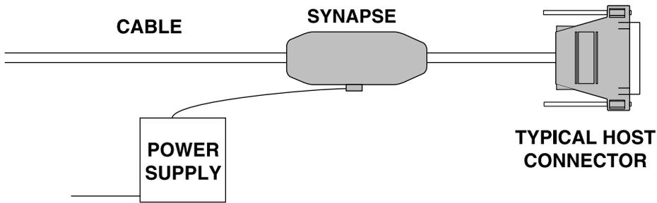
Figure 1-1. RS-232C External Power Connection using Synapse Cable
