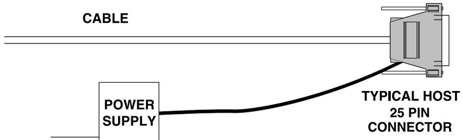
Figure 1-3. RS-232C External Power Connection: 25-pin Host Connector
