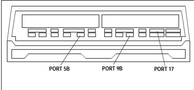
Figure 1-6. IBM 4683 Rear Panel with Cover Removed
