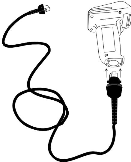
2. Twist the cable to the left to lock in place, as shown below:
