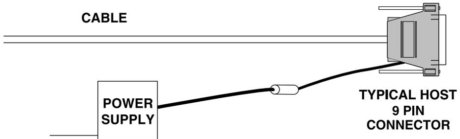
Figure 1-2. RS-232C External Power Connection: Flying Lead Connector to a 9-pin Host Connector
