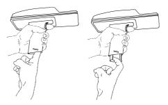
Figure 6-3. Removing the Alkaline Battery Adapter
