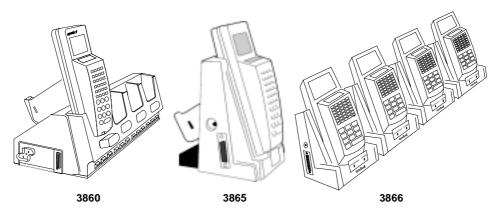
Figure 6-2. Charging the Battery in the Cradle
