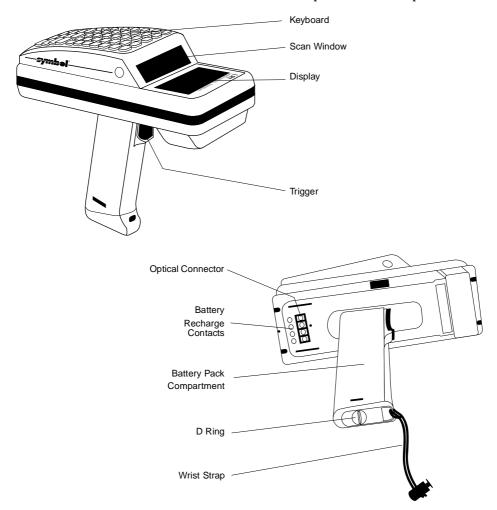
Figure 1-1. Series 3800 Terminal Parts
