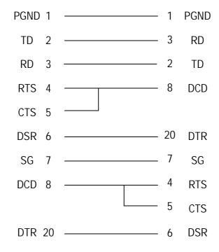
Figure A-2. Null Modem Pin-Outs - Half Duplex
