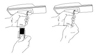
Figure 6-5. Installing the Alkaline Battery Adapter
