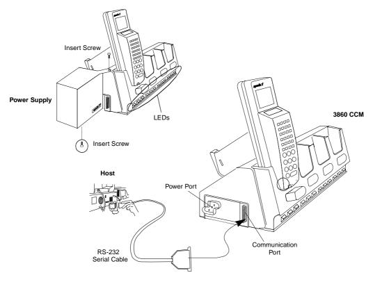
Figure 2-7. Connecting the 3860 CCM for Charging and Communications
