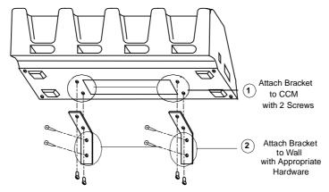
Figure 2-5. Wall Mounting the 3860 CCM
