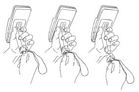
Figure 6-1. Removing the Battery Pack
