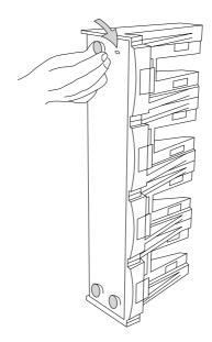
Figure 2-2. Installing Suction Cups on the CRD 3866
