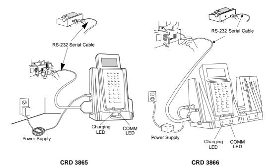
Figure 2-4. Connecting the 3865 and 3866 Cradles for Communications with Computer, Printer, or Modem
