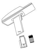
Figure 6-4. The Alkaline Battery Adapter
