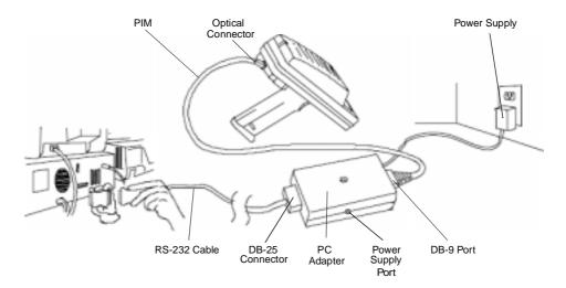
Figure 2-10. Setting Up the PC Adapter
