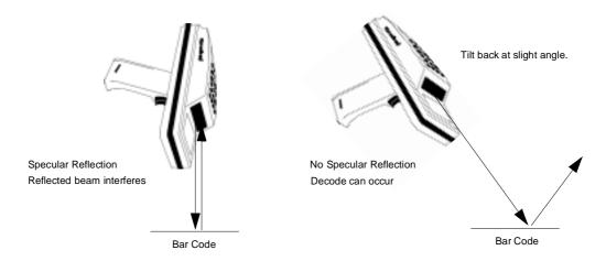
Figure 5-3. Scanning Angle and Specular Reflection
