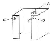
Figure 2-1. Wall Mounting the 3865
