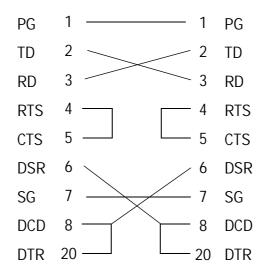
Figure A-1. Null Modem Pin-Outs - Full Duplex
