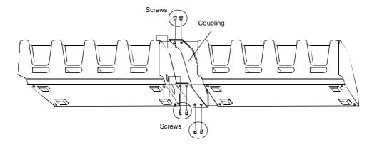
Figure 2-6. Coupling two 3860 CCMs
