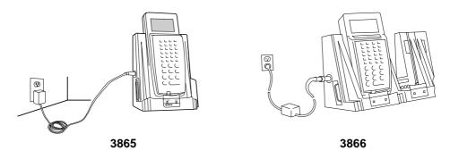
Figure 2-3. Connecting the CRD 3865 and CRD 3866 to a Power Source
