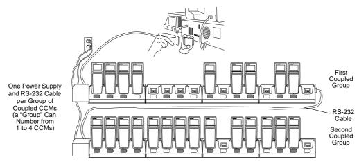
Figure 2-8. Daisy-Chaining Multiple 3860 CCMs
