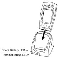
3. The Terminal Status LED turns red to indicate charging, then green when the battery is fully charged.
