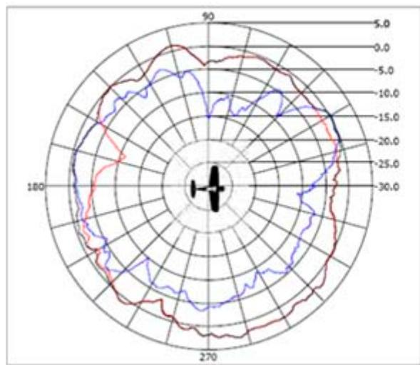
Azimuth Pattern 2436 MHz
