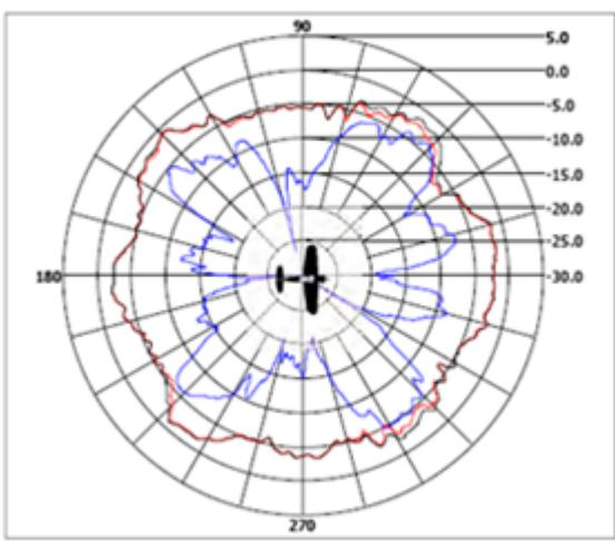
Azimuth Pattern 5500 MHz
