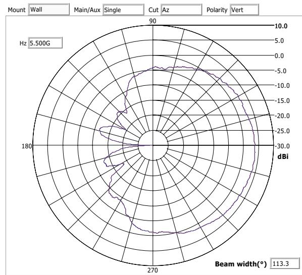
**Azimuth Pattern 5500MHz**
