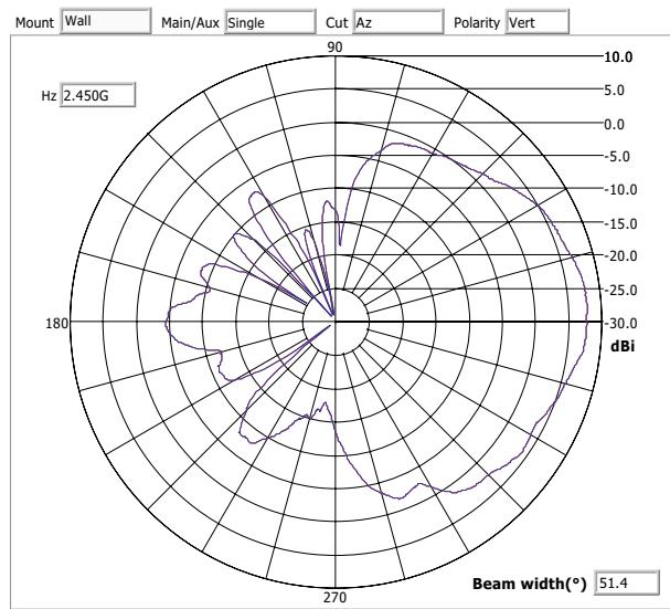
**Azimuth Pattern 2450 MHz**
