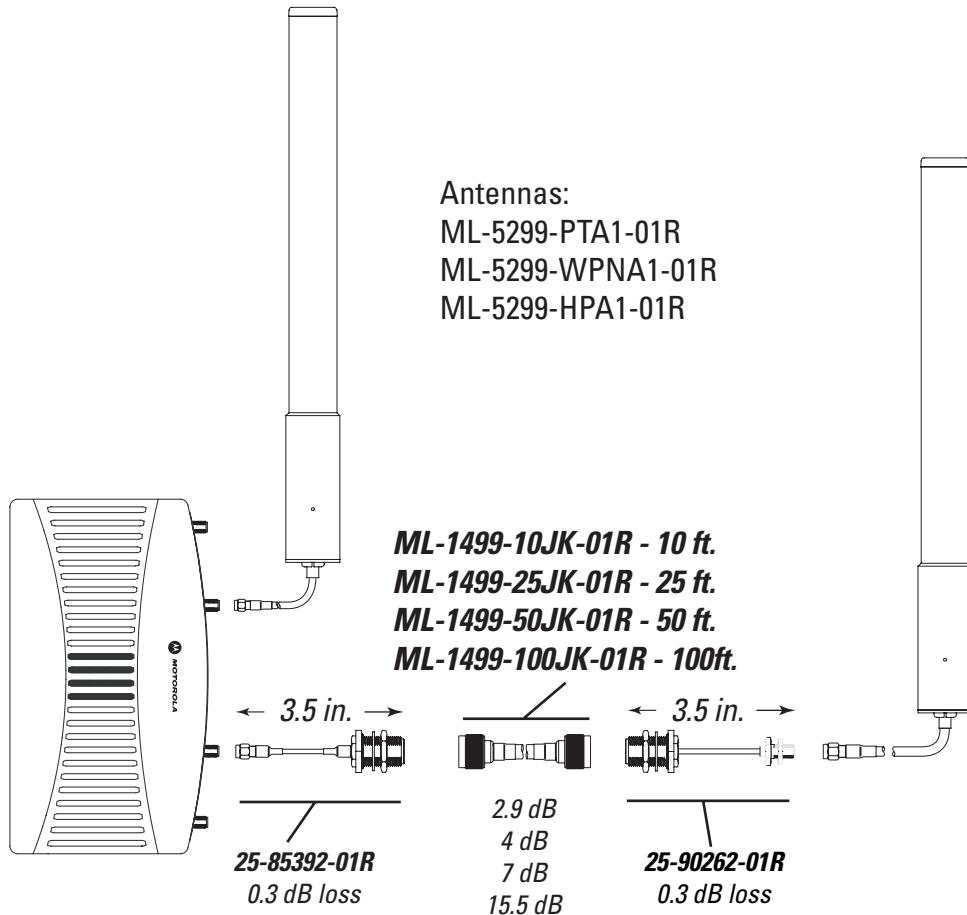
Refer to the following for a graphical depiction of the parts and connection options available for cabling an 5 GHz AP-5131 model access point using a RP-SMA male antenna (with a lightning arrestor):
