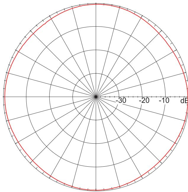
**Azimuth Pattern 5500 MHz**
