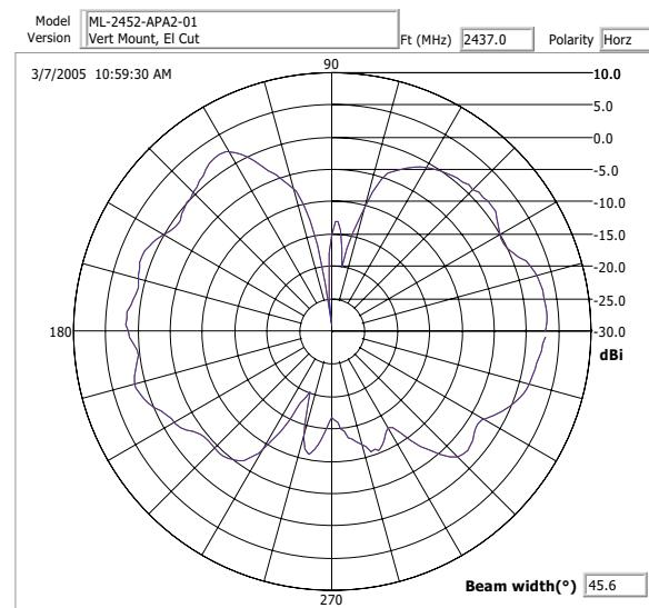
**802.11b Band****Elevation Pattern**
