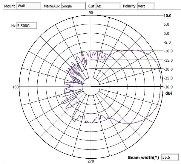
**Azimuth Pattern 5500MHz**
