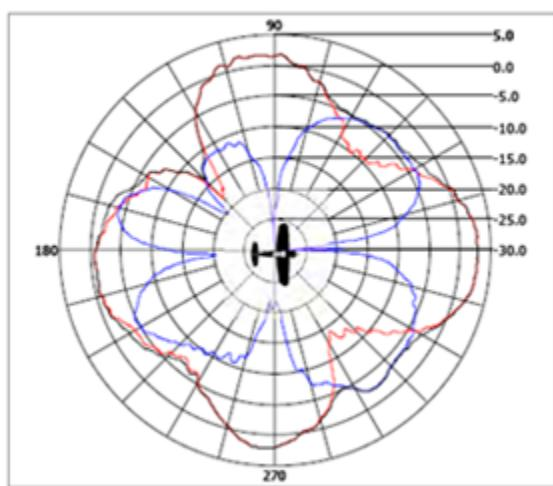
Azimuth Pattern 2436 MHz
