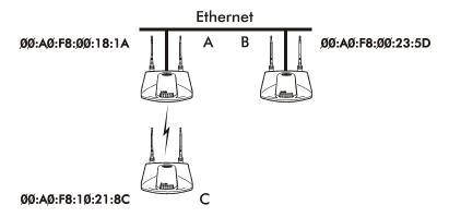
If an AP functions as a bridge between wired LANs, Symbol recommends one LAN contain all the lower WLAP IDs.
