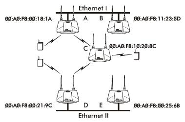
In this configuration, the WLAP Priority value is the default 8000 Hex. On concatenating this value to the MAC addresses of the APs, AP A on Ethernet I has the lowest WLAP ID with 800000A0F800181A, making it the Root AP. AP C uses the AP A channel, DTIM and TIM interval.
