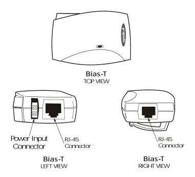
At the HUB end an Ethernet patch cable connects to the DATA port on the BIAS-T and DC power is connected using a DC power plug. The data signal and DC are combined within the BIAS-T and connected to the CABLE port. An additional patch cable connects the CABLE port to the Ethernet infrastructure. Use an Ethernet 4-pair patch cable to connect the individual access points to the BIAS-T power distribution system.
