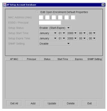
The AP Setup Account Database dialog box displays. Select the Edit Open Enrollment Default Properties checkbox.
