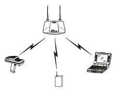
• A single AP can bridge the Ethernet and radio networks.
