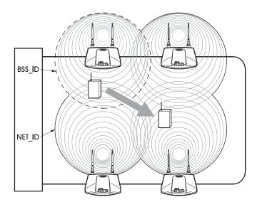
APs with the same Net\_ID (ESS) define a coverage area. The MU searches for APs with a matching Net\_ID (ESS) and synchronizes with an AP to establish communications. This allows MUs within the coverage area to move about or *roam*. As the MU roams from cell to cell, it switches APs. The switch occurs when the MU analyzes the reception quality at a location and decides which AP to communicate with based on the best signal strength and lowest MU load distribution.
