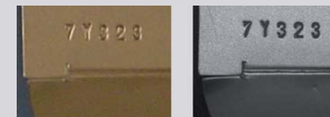
Object: Stamped characters on a metal plate. High contrast image allows inspection or reading.
