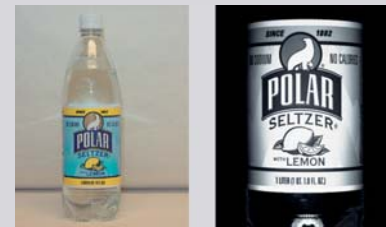
Object: Labeled bottle. Inspect for label presence or absence, correct label and proper orientation.
