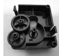
Gear arrangement for 305dpi
