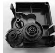
Gear arrangement for 203dpi
