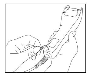
Figure 1. Disconnecting the Interface Cable
