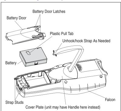
Figure 4. Installing the Battery Pack
