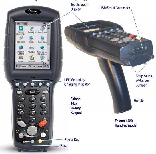
Figure 1. Falcon 26-Key Keypad and Connector Views
