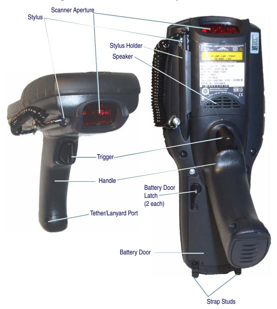
Figure 2. Falcon Scanner and Battery Door Views
