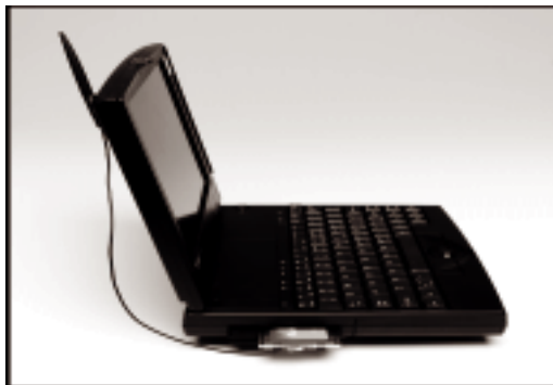
Figure 2 RangeLAN2 7400 Installation with Dipole Antenna
