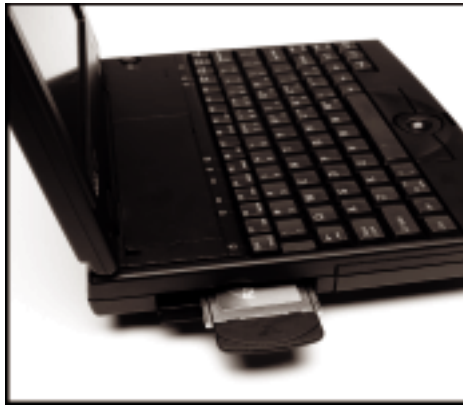
Figure 3 RangeLAN2 7400 Installation with Snap-On Antenna
