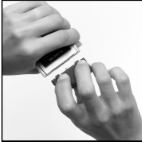
Figure 4 Pressing the Buttons for the Snap-On Antenna (Back of Card and Back of Antenna Shown)
