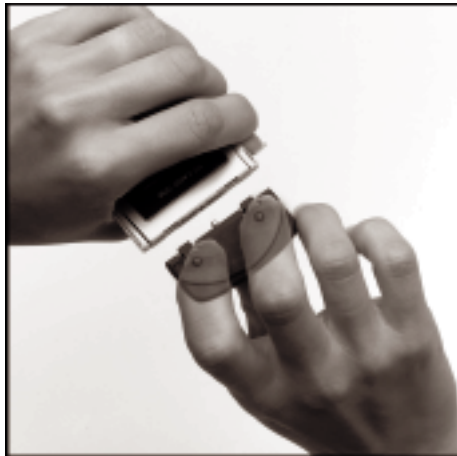
Figure 5 Pressing the Buttons for the Snap-On Antenna (Back of Card and Back of Antenna Shown)
