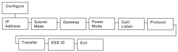
The Configure menu allows you to set the printer's IP Address, Subnet Mask, Gateway, Power Mode, Call/Listen, Protocol, Transfer, and ESS ID.
