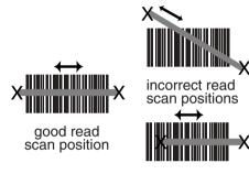
When reading a small bar code, decrease the distance between the terminal and the bar code. For larger bar codes, position the terminal so that the bar code fits into the laser beam. When reading a very high density bar code, decrease the distance between the terminal and the bar code. For a low density bar code, increase the distance between the terminal and bar code.
