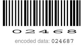
Fig. C.25. Example for S-Code
