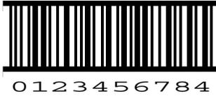
Fig. C.30. Example for MSI/Plessey with MOD 10 Checksum
