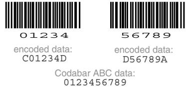
Fig. C.22. Example for Codabar CX
