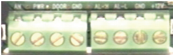
Figure 8: Cradle's screw terminals
