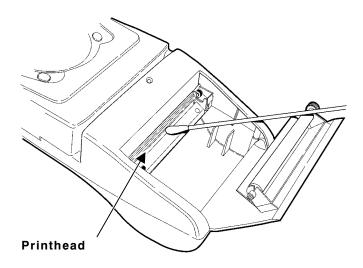
4. Clean the platen roller with a dry cloth or small brush. You can also use another cotton swab moistened with isopropyl alcohol. Turn the platen roller with your finger and run the cotton swab or dry cloth across it. Make sure the platen roller is clean all the way around.
