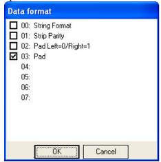
**Block Mode** – Click on .... to open up selection box. Click on check box to set or clear the desired bit. The Serial Status byte uses bits 0 through 6. Ignore bit 7.
