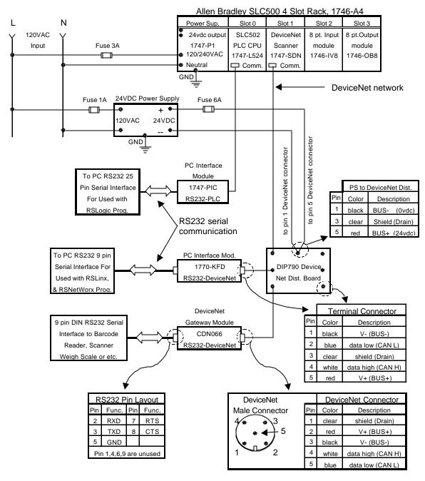
Figure 1. CDN066 Integrated with Allen Bradlev SLC500
