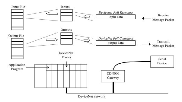
The CDN060 configuration defines the number of output bytes in a Poll Command message, and the number of input bytes in a Poll Response message. Each Poll Command and Poll Response message can contain up to 2 overhead bytes for CDN060 status and data synchronization information. The remaining bytes contain output data to be transmitted out the serial channel, or input data received by the serial channel.
