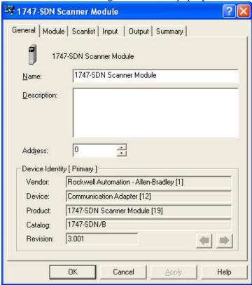
3) Select the Scanlist tab. RSNetworx prompts you for the Scanner Configuration. Click Upload to upload current 1747-SDN configuration from the node. RSNetworx displays the upload progress.
