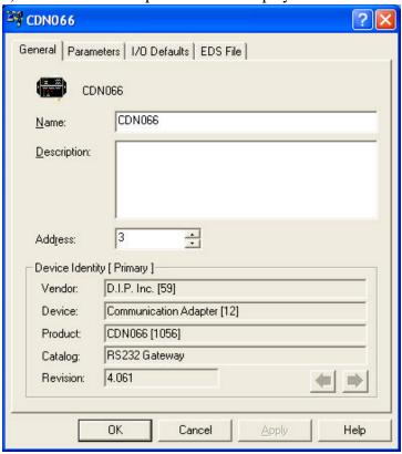
7) Select the *Parameters* tab. You will be prompted for the parameters source. Select the *Upload* button to upload CDN066 parameters from the actual device. All the CDN066 parameters are now shown in the *Properties* window.
