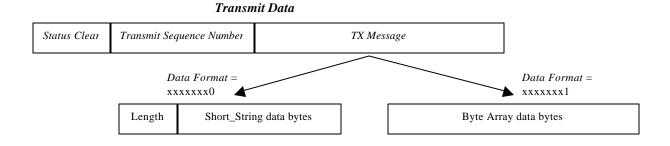
*Status* – Contains bit-mapped serial channel status and error bits for transmit and receive operations. Clearing the bits indicated will clear the error condition.
