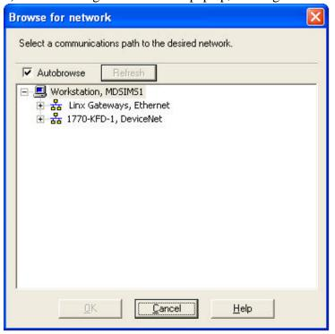
3) Click on the 1770-KFD-1 + to show all connected DeviceNet devices. The gateway is at MAC ID 03, verifying its DeviceNet connection. It is an *Unrecognized Device* until the gateway's EDS file is registered with RSNetworx.
