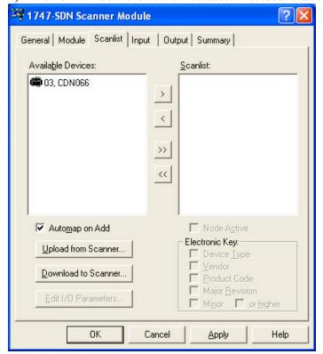
5) Select the Automap on Add checkbox if you want RSNetworx to automatically map the CDN066 input and output bytes into the 1747-SDN memory.
