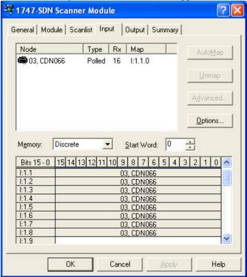
11) Click the *Advanced*... button to view current input mapping detail. Change the mapping to suit your application. Click *Apply Mapping* button after you make changes. Click *Yes* at the RSNetworx prompt to download any changes to the 1747-SDN. Click *Close* to continue.
