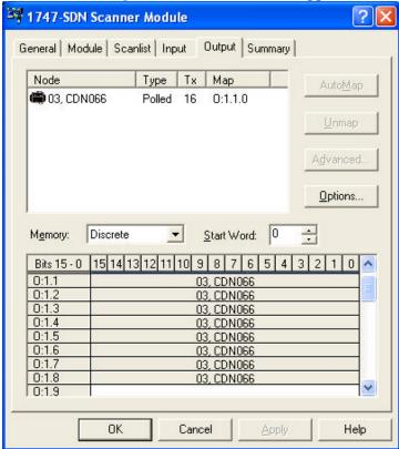
13) Click the *Advanced*... button to view current input mapping detail. Change the mapping to suit your application. Click *Apply Mapping* button after you make changes. Click *Yes* at the RSNetworx prompt to download any changes to the 1747-SDN. Click *Close* to continue.
