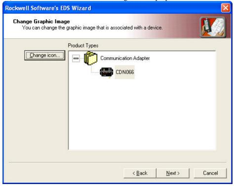
12) The final step is to finish EDS file registration. Click *Next>* to complete the registration process. Click *Finish* to close the EDS Wizard window.
