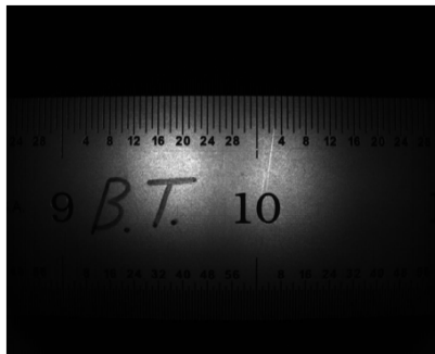
FIGURE 3–2. Off-Axis – Semi-Specular Surface (Fine Matte Metal Ruler) at 2”, Optical Axis of Camera Positioned at 60° from Image Plane
