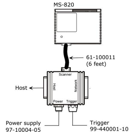
Figure A-3 Scanner/IB-131 Typical Setup
