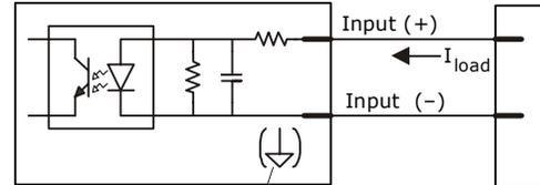
New master pin input (-) is internally grounded.
