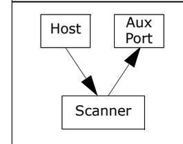
**Usage:** Useful when the user wants bar code data displayed on an auxiliary screen close to the scanner.
