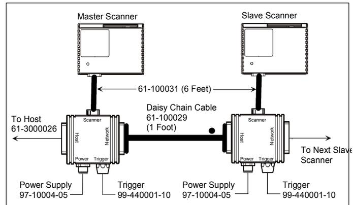
Figure A-5 Scanner/IB-131 Daisy Chain Setup
