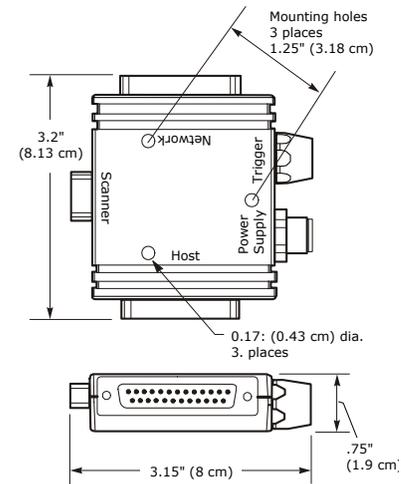
Figure A-2 IB-131 Mechanical
