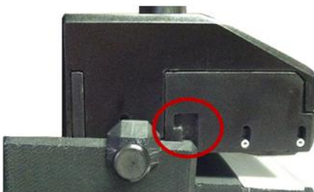
Align the readhead's L-shaped slot on the docking plate lip.
