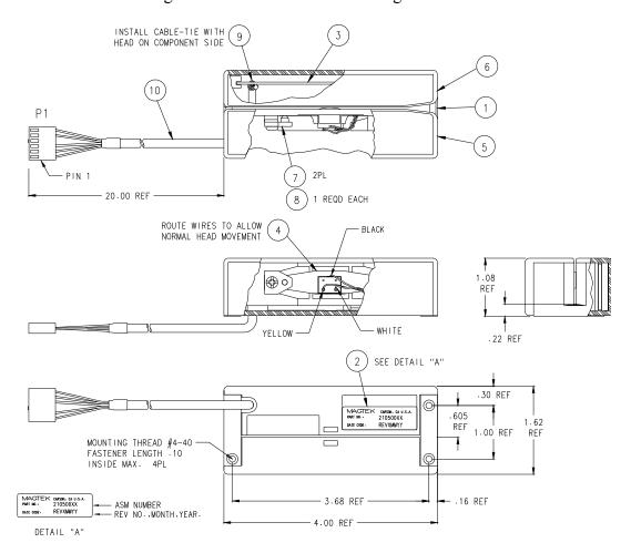
Figure 2-1. Reader Mounting Dimensions With Cover
