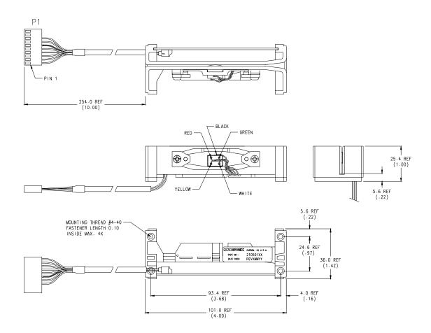
Figure 2-2. Reader Mounting Dimensions Without Cover
