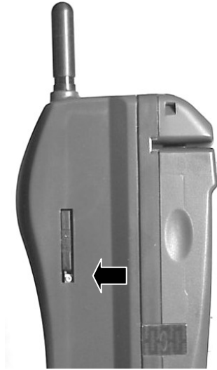
Figure 10: Left side of LP 9100 GPRS terminal showing the SIM tray inserted. The arrow points to the yellow ejection button on the lower end of the tray.
