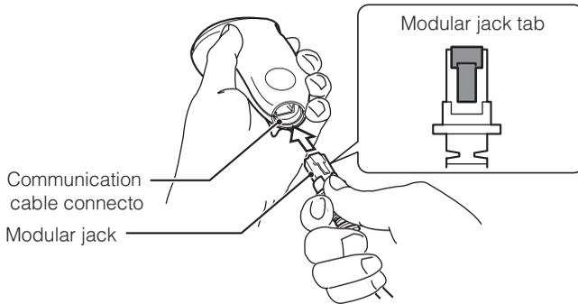
Gently pull on the cord protector for the connection cable to verify that it is locked into place. Connection is complete.
