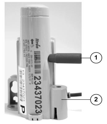
For an 80W-i endpoint, insert the tip of the pen magnet (1) into the depression beside the screw hole (2) and touching the blue tamper seal. Hold the magnet perpendicular to the endpoint housing for four seconds, and then remove it.
