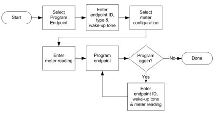
You can use the **Program Endpoint** command option with 40W, 50W, 60W, and 80W-i endpoints. An FC200SR or FC300SR handheld or a laptop with a 900MHz belt-clip radio is required for 60WP and 80W-i endpoints.
