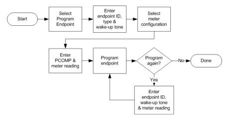
You can use the **Program Endpoint** command option with all ChoiceConnect 40G/GB and 100G series gas endpoints. An FC200SR or FC300SR handheld or a laptop with a 900MHz belt-clip radio is required with 100G series endpoints.
