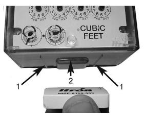
• Place the magnet face with the Itron logo and part number flat against the bottom of the cover, with the arrow on the magnet pointing toward the back of the module. Slide the magnet back toward the 2.4GZ back plate until it touches the stop. Hold the magnet in place for five seconds and remove it.
