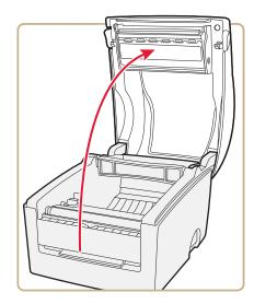
**2** Pull or lift the spindle and insert a fresh media roll onto the spindle. If you are replacing a roll of media, remove the empty label roll core and insert the new media roll onto the spindle.
