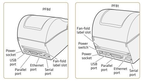
PF8d and PF8t Rear View Connections and Controls
