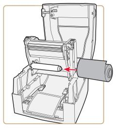
**4** Insert a new transfer ribbon roll onto the ribbon supply shaft.
