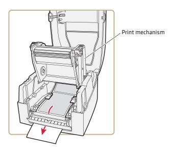
Threading the Liner Inside the Peel-off Mechanism for PF8t
