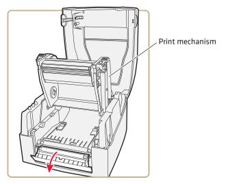
Opening the Self-Strip Mechanism on the PF8t
