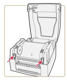
**3** Insert the empty ribbon take up core onto the ribbon rewind wheel. Make sure that the cardboard spindle is attached to the core.
