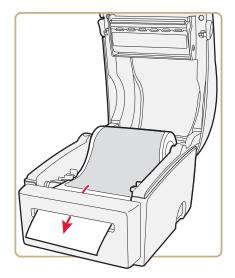
Routing the Liner Inside the Cut-off Mechanism for the PF8d
