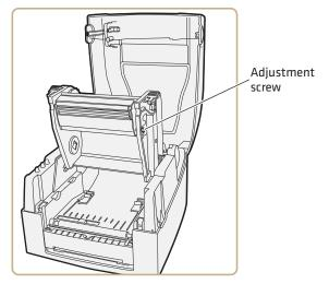
PF8t Printhead Alignment Adjustment Screw
