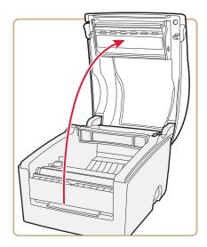
**2** If you have a PF8t, press the locking mechanism and open the print mechanism and ribbon container to load media and access the media adjustment tabs.
