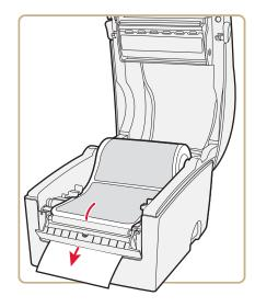
Threading the Liner Inside the Peel-off Mechanism for PF8d
