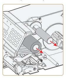
**4** Slide the ribbon roll onto the supply hub so the ink-coated side faces down when the ribbon is routed through the print mechanism.
