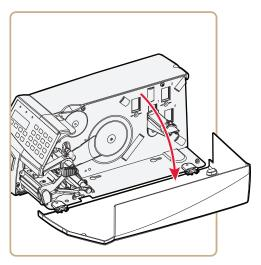
**2** To raise the printhead, turn the printhead lift lever clockwise.
