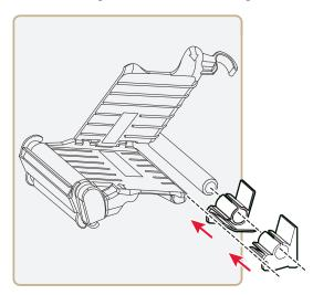
**7** Slide the inner guide as far as possible down the shaft so that it is flush with the center section.
