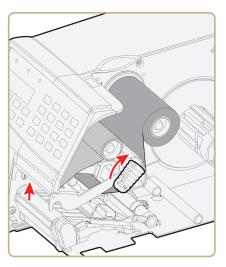
**4** Remove any empty core from the media supply roll post.
