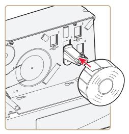
**4** If necessary, adjust the outer quick-load guide to fit the width of the media.
