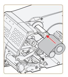
**5** Route the ribbon through the print mechanism above the transparent upper LSS guide and pull out approximately 20 cm (8 in) of ribbon leader.
