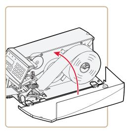
**9** Press the **Print** button to advance the media and adjust the media feed. Tear off the media by pulling it downwards.
