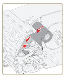
**10** Turn the printhead lift knob counterclockwise to engage the printhead.
