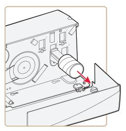
**4** Fit a new roll of media on the supply hub. Adjust the edge guide so the roll becomes flush with the center section.
