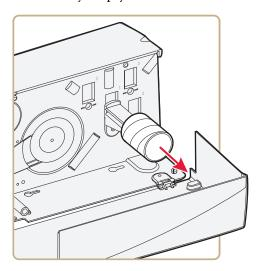
**3** Fit a new roll of media on the supply post. Adjust the edge guide so the roll becomes flush with the center section.
