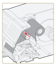
**8** Turn the printhead lift lever clockwise to raise the printhead and release the ribbon.
