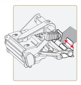
**5** Insert the media between the guides and feed the media forward until it reaches the platen roller and stops.
