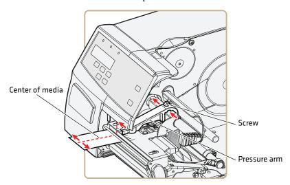
**4** Move the pressure arm inward or outward until the arrow on the tip of the arm is centered with the media.
