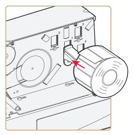
**6** Route the media through the print mechanism and cutter. Then, push it towards the center section as far as it will go.
