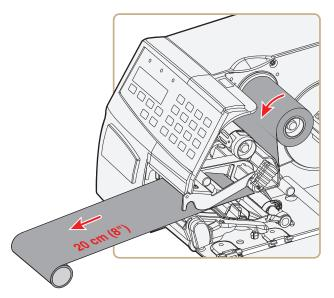
**6** Without releasing the ribbon, turn the printhead lift lever counterclockwise to engage the printhead and lock the ribbon.
