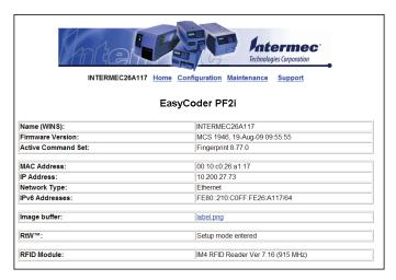
The home page displays the assigned name, firmware version, Active Command Set, MAC address, and IP address of your printer. The home page also displays the contents of the image buffer, as well as the status of the Ready-to-Work indicator.
