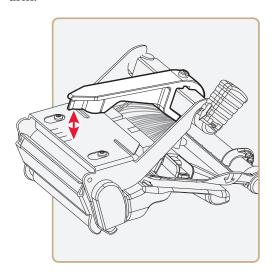
**6** Disconnect the printhead bracket from the print mechanism, and pull out the printhead as far as the cables allow.
