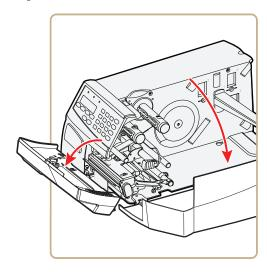
**3** Turn the printhead lift lever clockwise to raise the printhead.
