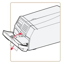
**11** Press the **Print** button to advance the media and adjust the media feed. The labels can be collected on an optional tray.
