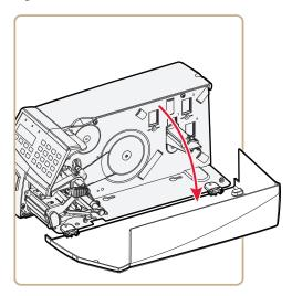
**3** Disengage the upper guide from the lower guide by lifting the inner part of the upper guide and pulling it out. Make sure not to damage the cable.
