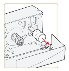
**5** Fit a new roll of media on the supply post. Fold up and adjust the edge guide so the roll becomes flush with the center section.
