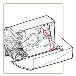
**2** Remove any empty core from the media supply roll post.
