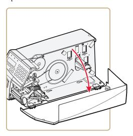
Disengage the upper guide from the lower guide by lifting the inner part of the upper guide and pulling it out. Make sure not to damage the cable.
