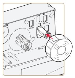
**6** Remove labels from the first 50 cm (20 in) of the liner. Route the liner through the print mechanism and push it inward toward the center section as far as it goes.
