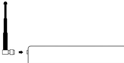
**Figure 5-1 Attachment of the Mercury antenna**
