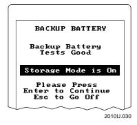
3. The Backup Battery screen appears, describing the status of the lithium bridge battery.
