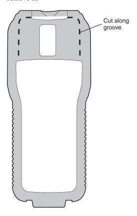
**2** Slide the top of the CK30 into the boot, and pull the bottom of the boot over the bottom of the CK30.
