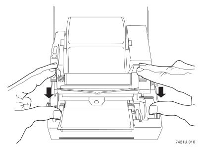
14. Activate the label taken sensor by pressing in on the top of the sensor. The printer is now ready for printing.
