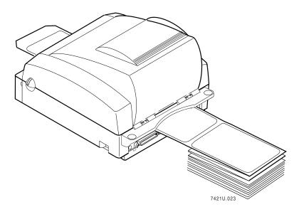
6. Center the labels in the printer path and adjust the label guides so that they just touch the edges of the label liner. Wind the yellow adjustment roller toward the rear of the printer.
