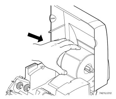
7. Insert the end of the roll into the printer and out the front of the printer.
