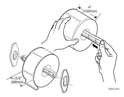
6. Place the roll inside the top cover so that the end feeds from the top.
