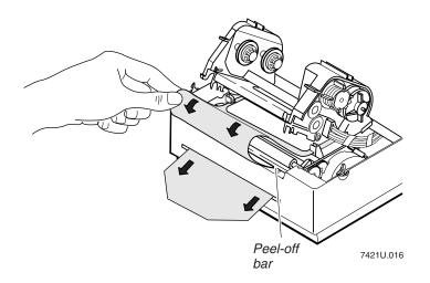
12. Pull the label liner out of the bottom slot until the liner is tight across the peel-off bar.
