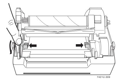
5. Insert the spindle into the roll of media.
