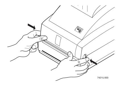
2. Open the printhead assembly by pulling the yellow release lever toward the front of the printer.
