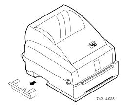
3. Insert the memory card, label side up, into the memory card slot. Push firmly to engage the memory card.
