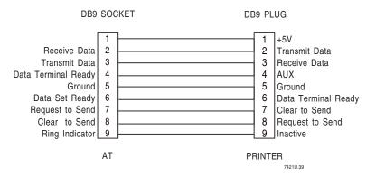
RS-232 Null Modem Cable for PC for 25-pin to 9-pin
