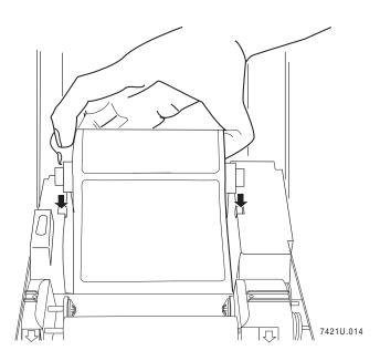
9. Center the labels in the printer path and adjust the label guides so that they just touch the edges of the label liner.
