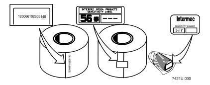
*Note:* Some ribbon rolls have the media sensitivity number printed on the inside core.
