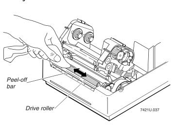
Cleaning the Drive Roller and Peel-Off Bar
