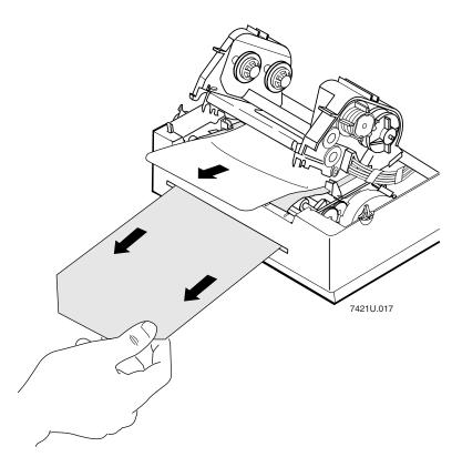
13. Lower the printhead assembly and lock it into the operating position by pressing down firmly on both sides of the printhead. Lower the printer cover.
