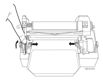
7. Lower the printhead assembly and lock it into the operating position by pressing down firmly on both sides of the printhead. Lower the printer cover.
