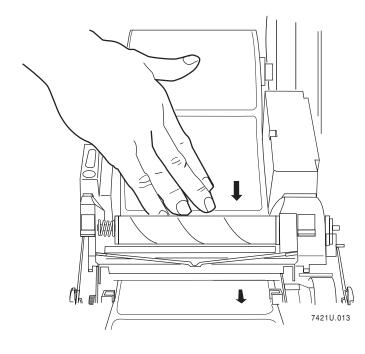
8. Rewind the excess paper onto the media roll while placing the spindle into the holder slots on the printer.
