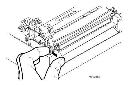
3. Lift the printhead up into the full open position.
