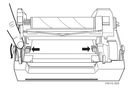
5. Place the fanfold media slightly lower than the slot in the printer back cover and insert the media through the slot, into the printer mechanism, and out the front of the printer.
