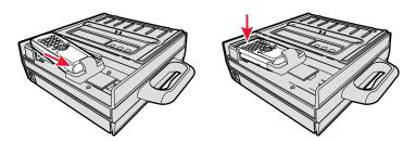
Inserting a Computer in a Terminal Holder
