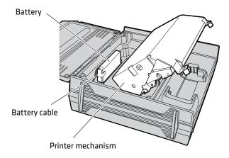
Installing the Internal Battery
