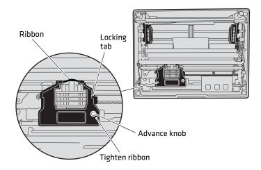
Installing the Ribbon Cartridge
