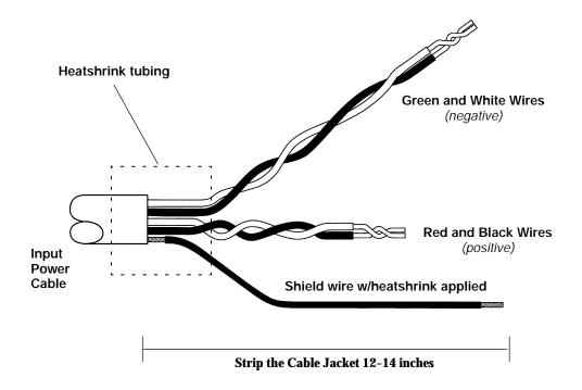
Figure 2-1 Cut and Strip Cable Ends
