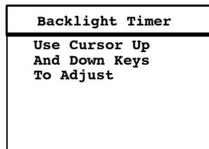
Use the up[▲] and down[▼] arrows to select a number from Off to 255. This is the number of seconds that the backlight stays on after a key is pressed.
