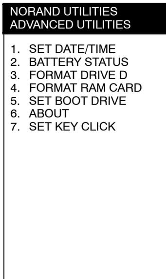
Press the number of an advanced utility option, or press the ▲ or ▼ keys to scroll through the list, then press the [ENT] key to enter.
