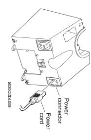
4. You can secure the dock to a flat surface using the two rear mounting holes and two #8 pan head screws (not provided). Do not overtighten.
