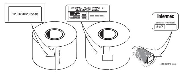
**MSN:** This illustration shows you where to find the MSN. Note that some ribbon rolls have the MSN printed inside of the core.
