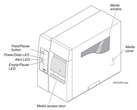
**4420 and 4440 front view:** This illustration shows the 4420 and 4440 features on the front of the printers.
