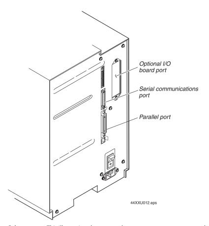
**Printer ports:** This illustration shows you where to connect your system to the printer.
