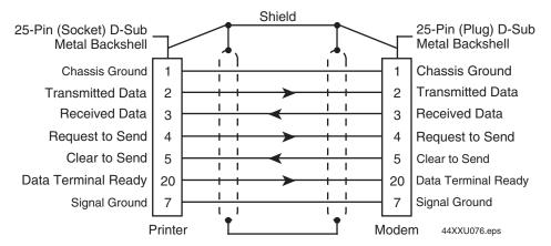
**Straight Through DTE to DCE Cable:** This illustration shows the pin assignments for the straight through DTE to DCE cable used with a modem (P/N 043237S). If you find that you are losing data, you may need to isolate the chassis ground from one of the two devices by connecting it to the shield.
