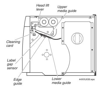
**6** Insert the cleaning card into the printer following the media path.
