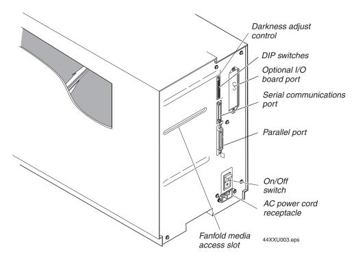
**4420 and 4440 back view:** This illustration shows the 4420 and 4440 features on the back of the printers.
