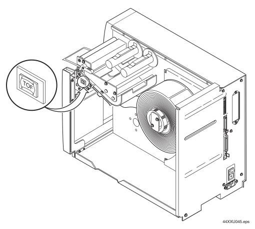
**TOF switch:** The TOF switch is a small rocker switch located on the lower outboard plate of the printer.
