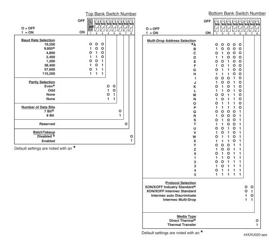
**DIP switch settings:** These charts illustrate the settings for the DIP switches on the top and bottom banks. For a description of each setting, see the DIP Switch Settings Descriptions table earlier in this chapter.
