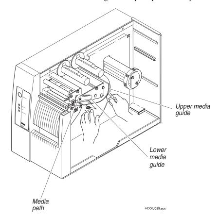
**5** Clean the lower media guide by using a lint-free cloth moistened with isopropyl alcohol as shown in the following figure.
