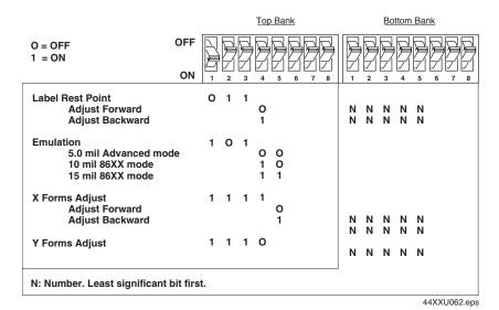
**Configuration DIP switch settings:** This illustration shows the Test and Service mode DIP switch settings for changing the configuration commands.
