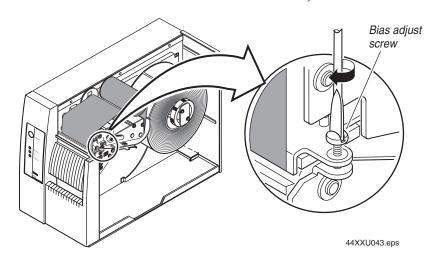
**2** To compensate for uneven print quality, use a straight-slot screwdriver to turn the bias adjust screw as shown.
