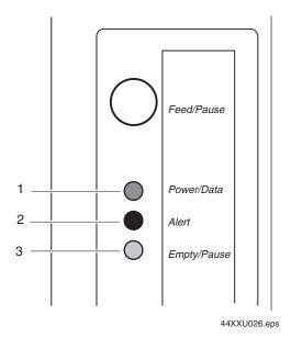
**Front panel LEDs:** This illustration shows the LEDs that are on the front panel of the printers. For help understanding these LEDs, see the next LED Descriptions table.
