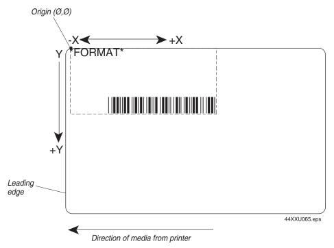
**Default X and Y origins:** This illustration shows the default X and Y origins. You can control the default X origin (top of form) with PrintSet or with the Test and Service DIP switches. You can control the default Y origin with the DIP switches only.
