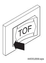
**3** Press the TOF switch repeatedly until the format moves backward to the correct position on the label.
