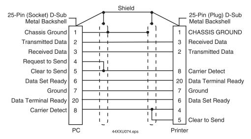
**25-Pin PC Connector RS-232 null modem cable:** This illustration shows the pin assignments for the RS-232 null modem cable for the 25-pin PC connector (P/N 048668).
