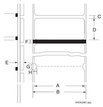
**Media dimensions:** This illustration shows to measure the media dimensions. See the next table, Minimum and Maximum Media Dimensions, for specific media dimensions.
