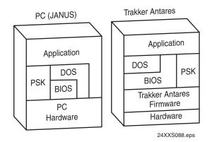
**DOS architecture:** This illustration compares the Trakker Antares DOS architecture to the JANUS (PC) DOS architecture. Use this diagram to understand the limitations of DOS on the terminal.
