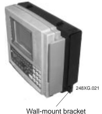
Intermec recommends that you use the desk or wall-mount bracket to mount the T248X and protect the power supply. You can use other mounting brackets or enclosures. However, without the Intermec desk or wall-mount bracket, the power supply is intended for indoor use only. Use of any other mounting brackets or enclosures will void the environmental protection ratings of the terminal.
