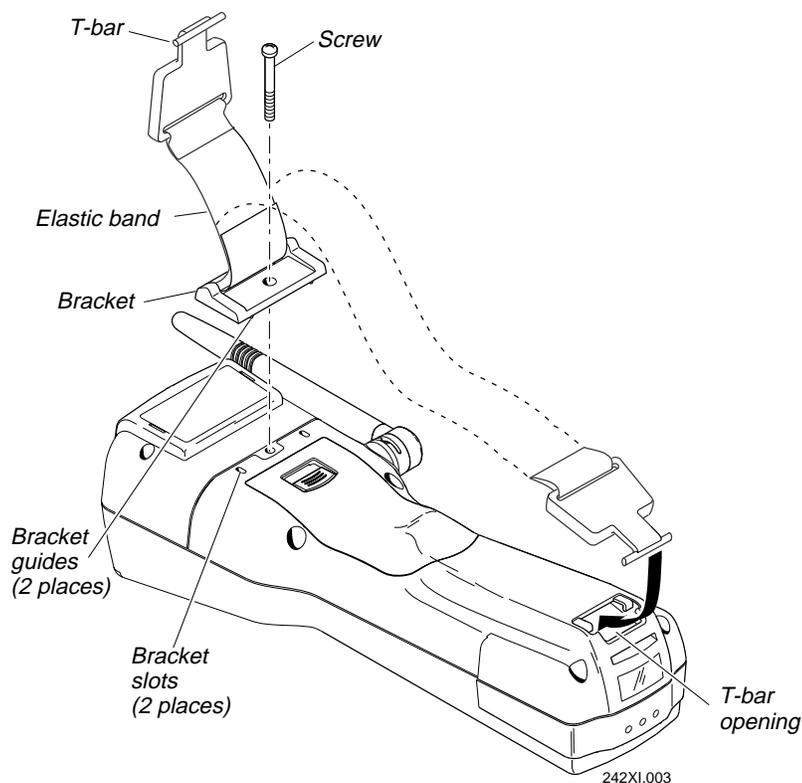
2. Align the handstrap bracket so the two bracket guides line up with the bracket slots on the terminal.
