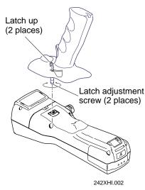
If the latch adjustment screws are difficult to insert, loosen the screws 1/4 turn counterclockwise. Repeat, if needed, until you can attach the handle.
