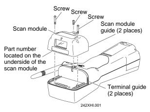
3. Locate the part number on the underside of the scan module. This handle works with the following scan modules only:
