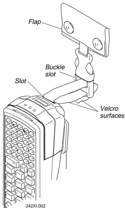
If you need to temporarily remove the terminal, squeeze the buckle to release it. To reattach the terminal, simply snap the buckle ends together.
