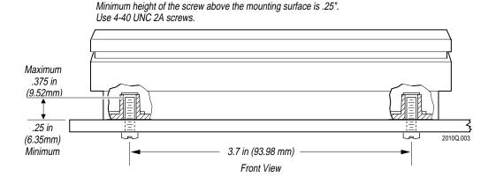
**Note:** If you mount the JZ2010 battery charger on a table top or shelf, make sure you have enough vertical clearance to insert and remove battery packs easily. Also remember to leave space behind the charger so that you can connect the power supply and reach the discharge button on the back panel.
