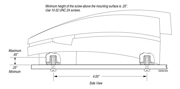
**Note:** If you mount the JD2020 communications dock on a table top or shelf, make sure you have enough vertical clearance to insert and remove the JANUS 2020 easily. Also remember to leave space behind the dock so that you can connect the power supply and reach the discharge button on the back panel.
