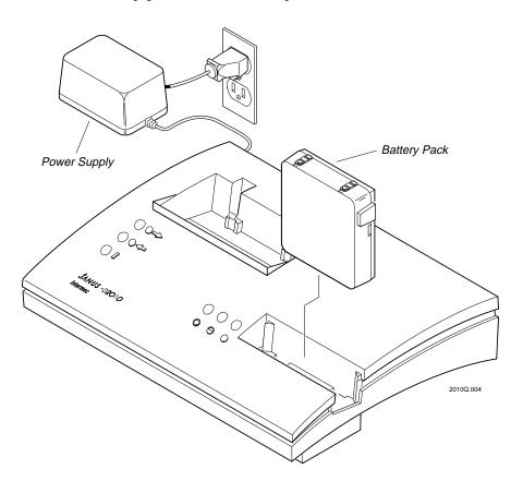
2. If you are charging a battery pack for the first time, the Charge LED flashes to indicate that the dock is precharging the battery. Once a battery pack has been precharged or if you have charged the battery pack before, the Discharge and Charge LEDs start flashing.
