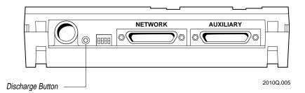
Insert the battery pack into the battery slot on the dock. The Discharge LED flashes and the communications dock begins discharging the battery pack. Allow several hours to completely discharge the battery pack.
