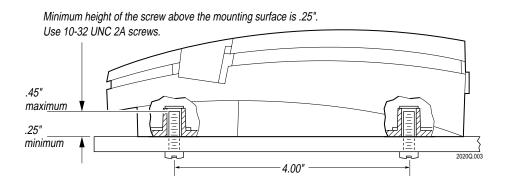
**Note:** If you mount the JD2010 communications dock on a table top or shelf, make sure you have enough vertical clearance to insert and remove the J2010 easily. Also remember to leave space behind the dock so that you can connect the power supply and, cables and reach the discharge button on the back panel.
