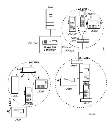
3. Physically connect the controller to your host environment. The Model 200 Controller supports Ethernet, token ring, coaxial, twinaxial, and SDLC networks using different local network adapter cards.
