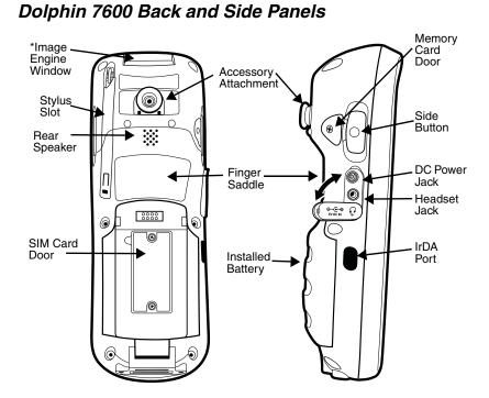
\*Pull the plastic tab to remove the plastic film cover over the image engine window before activating the image engine.
