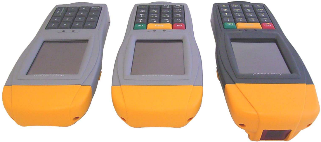
Fig. 1: Laser scanner (Option S5) – Imager with laser aimer (Option S6) – Long range scanner (Option S2)
