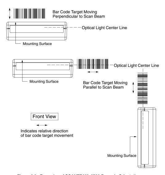
Figure 3.3 Examples of SCANTEAM 3700 Barcode Orientation
