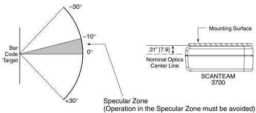
Figure 3.5 Specular Reflection Interference
