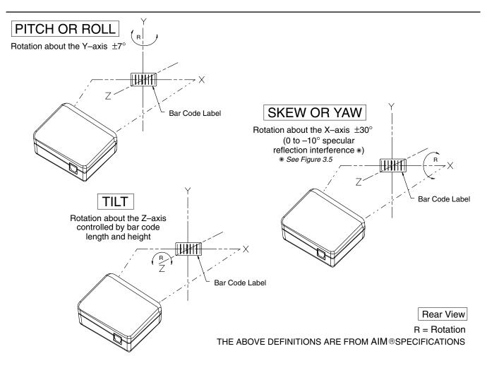
Figure 3.4 SCANTEAM 3700 Pitch, Skew and Tilt Tolerance
