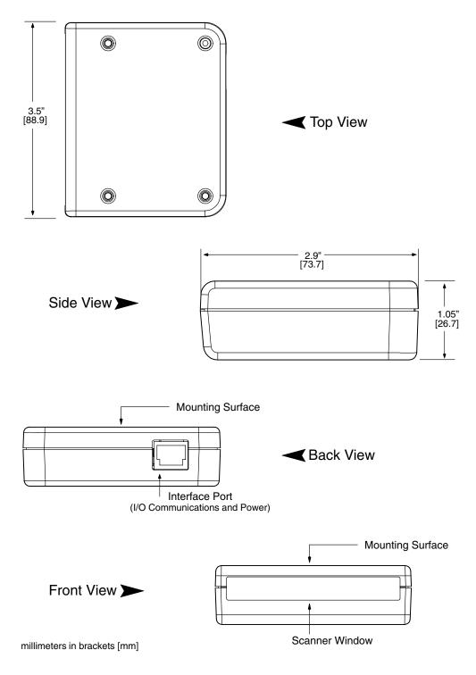
Figure 2.2 3700 Fixed Mount CCD Dimensions
