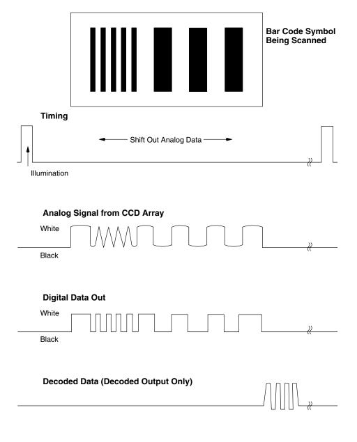
Figure A.2 SCANTEAM 3700 Timing Sequence
