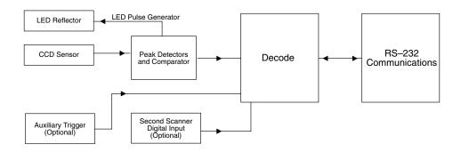
Figure 2.3 Basic Scanner/Decoder Operation
