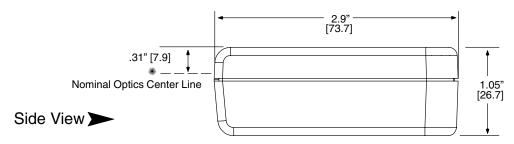
Installation should provide adjustment to align the optical center line on the intended target. This adjustment should account for tolerance variation in the 3700 scanner, as well as the host equipment.
