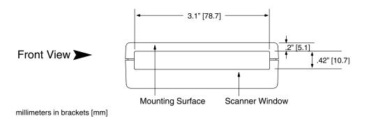
Figure 3.2 Mounting Dimensions for the 3700
